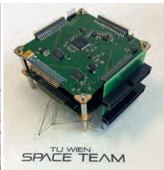
1:1 model (left) and On-board Computer of the Pegasus satellite.
